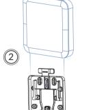
Slide the Access Point over the mounting plate.
