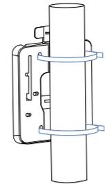
Slide the cable ties through the mounting plate and fasten them around the pole.
