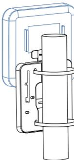
Slide the Access Point over the mounting plate.
